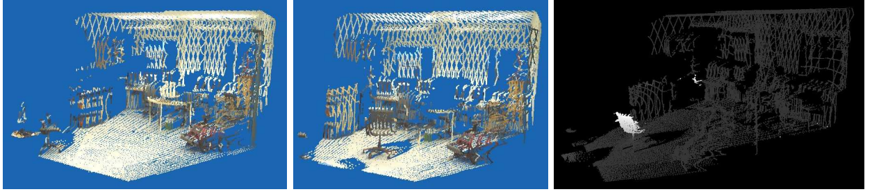
Fig. 2. Left, middle: 3D range scans recorded at a relatively small displacement of approx. 1 m. Right: Difference probability corresponding to a chair that was placed in the scene before the second scan was recorded. Brighter regions indicate a higher difference probability.
