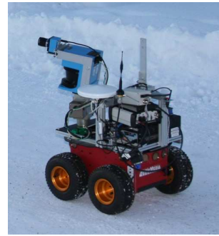
Fig. 5. Our mobile robot platform “Tjorven” equipped with the sensors used in this paper: the SICK LMS 200 laser range scanner and a colour CCD camera both mounted on an Amtec pan tilt unit.
