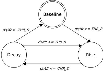
Fig. 3. Finite State Machine that illustrates the segmentation algorithm.
