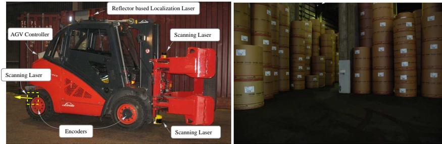
**Fig. 4** Left: The industrial truck used. The truck is retrofitted with an AGV controller. The bottom lasers are used as safety sensors and in this work also for landmark detection. Right: Stacked paper reels waiting to be loaded and one of the concrete pillars.
