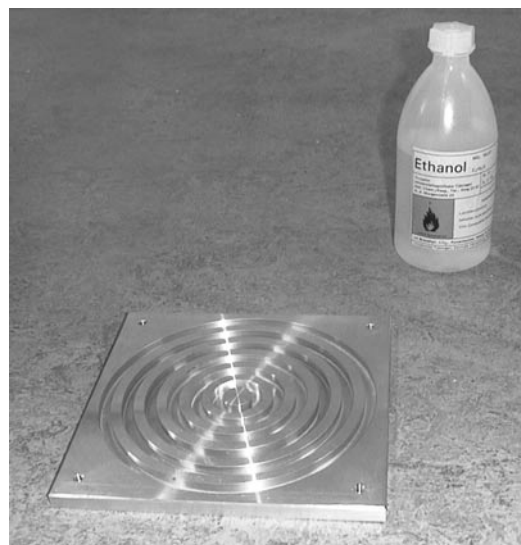
Figure 5: Vessel used as an odour source, that the robot is able to drive over without wetting its tyres by picking up the chemical. It is made of a square aluminium plate (having a width of 18.4cm ) in which six nuts ( 7mm wide, 7mm deep) were milled along concentric circles of the radii 1.25cm , 2.55cm , 3.95cm , 5.35cm , 6.75cm and 8.15cm respectively. Thus offering surfaces of 5.5cm^2 , 11.2cm^2 , 17.3cm^2 , 23.5cm^2 , 29.7cm^2 and 35.8cm^2 , which adds up to a maximum total amount of 123.2cm^2 (equal to a jar with a diameter of 12.5cm ).
