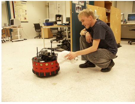
Fig. 6. (Left) Human presenting an odourous object (Right) The trace of the robot's movement during the search for an object of a particular odour in a room containing gasbottles, suitcases, boxes, and other objects.
