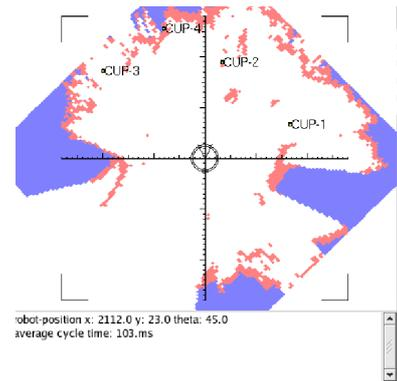
Figure 4: The local perceptual space of Pippi given 4 similar cups and obstacles. Pippi is located in the center of the space.
