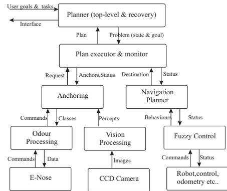
Figure 1: Overview of the robotic complete system which uses an anchoring module. On the left side of the arrows information is flowing downward and on the right side information is flowing upward.
