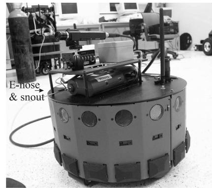
Figure 3: A closer view of the Pippi and the electronic nose.
