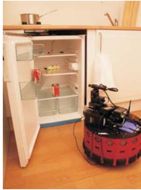
Figure 7: A future prospect for artificial olfaction for an intelligent environment. By tagging objects with RFID tags and using information about their properties a mobile robot with an e-nose can better constrain the classification context in order to improve performance. In this example, Pippi could be used to better inspect objects with the e-nose inside a refrigerator after a simple alarm has been generated.
