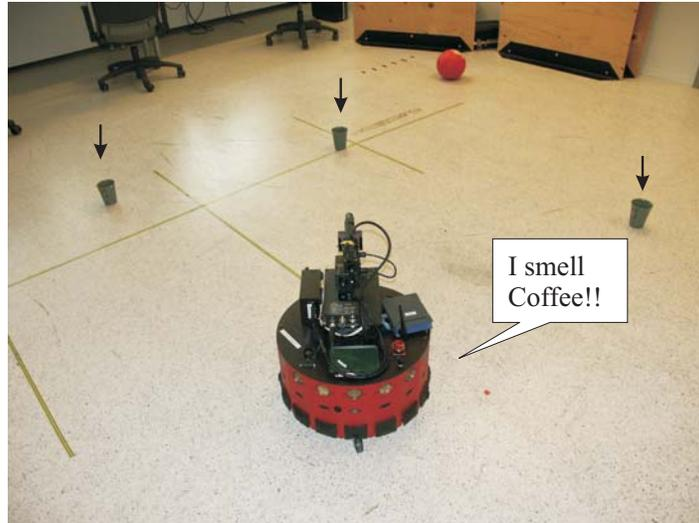
Figure 3: A situation where active sensing may be needed. Here the robot in the middle of the image detects an odor using the gas sensors but sees several candidate odor sources. Planning can be used to first approach each candidate and then actively engage a thorough odor sampling process in order to determine the character of each object and resolve the ambiguity.
