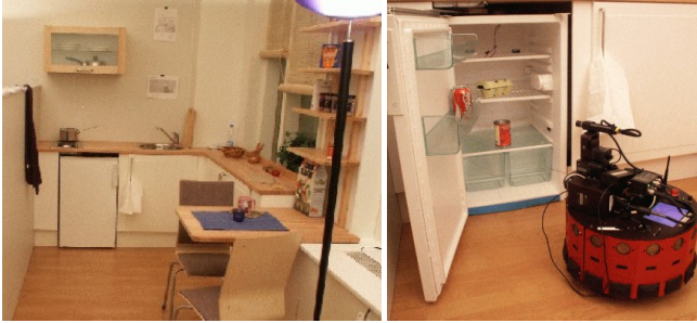
Figure 4. The experimental test-bed, the PEIS-room: view of the kitchen, and robot inspecting the fridge with video camera and electronic nose.
