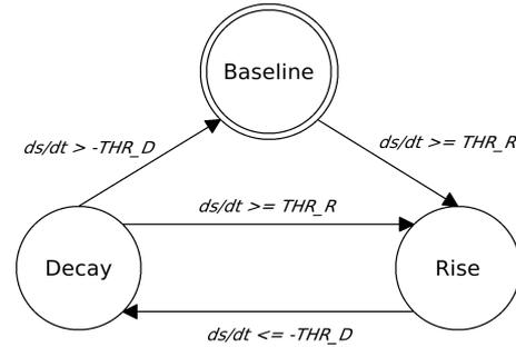
**Figure 2.** Finite State Machine that illustrates the segmentation algorithm.
