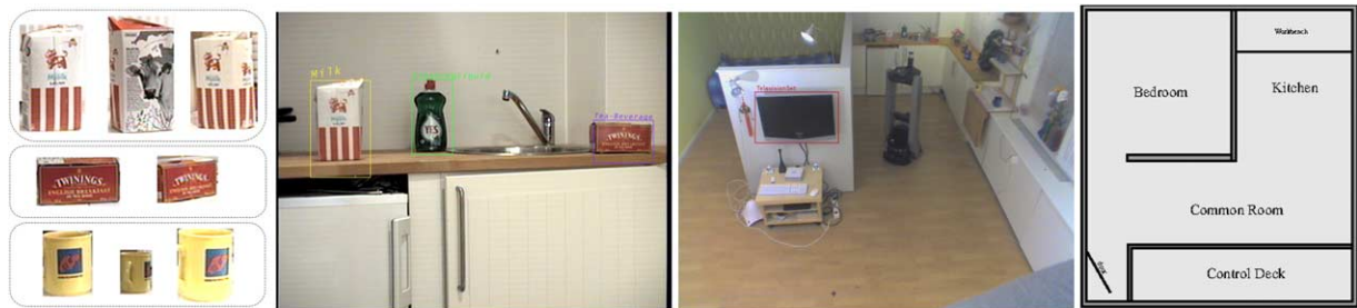
Fig. 6. From left to right. Sample training images of objects. The robot's perceptual space with the visually recognized objects. Similarly, ceiling camera's perceptual space. The PEIS-home Symbolic Map.
