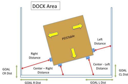
Fig. 7. Illustration of the relevant quantities used in the fuzzy rules for precision docking.
