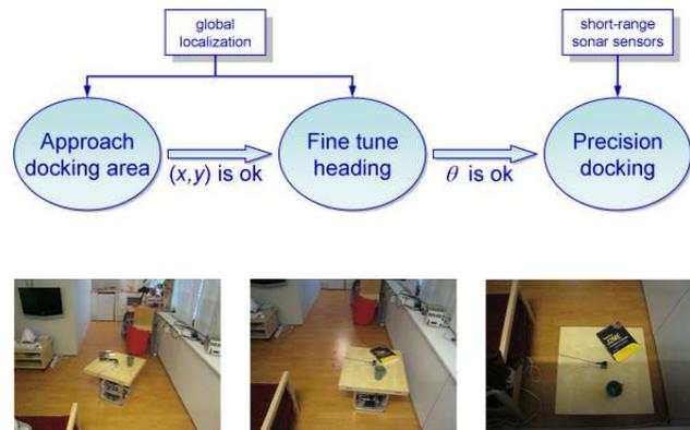
Fig. 6. The three steps of the docking behavior.
