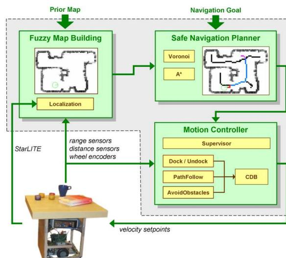
Fig. 2. Schematic control architecture of the PEIS-Table.
