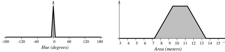
**Fig. 3.** Fuzzy sets for hue (left) and area (right) obtained from the vision system.
