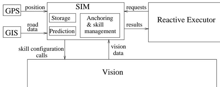
**Fig. 1.** Overview of the Scene Information Manager and its interaction with the Vision module and the Reactive Executor.
