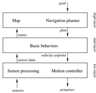
**Fig. 4.** Hierarchical structure of the control software
