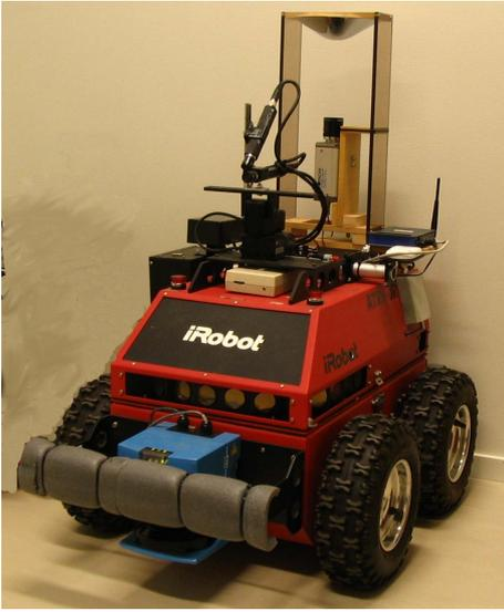
Fig. 4. The ATRV-Jr research robot used to evaluate the mine navigation system.
