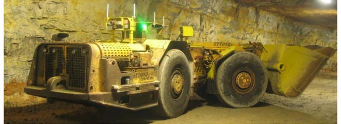
Fig. 1. LHD vehicle prepared with sensors and control system for autonomous navigation.
