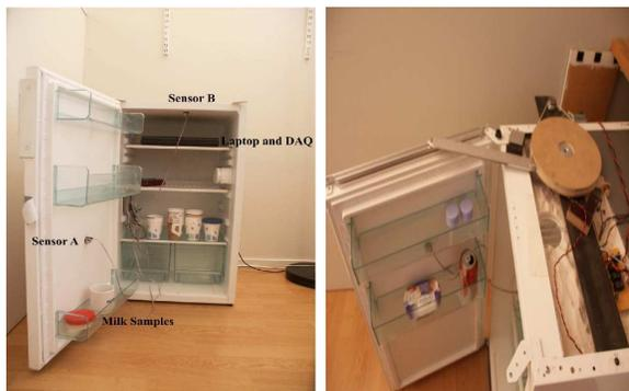
Fig. 3. (Left) The PEIS fridge showing the placement of the two gas sensors and the products to be sampled (Right) The door mechanism which opens and closes the fridge door.
