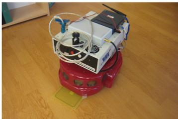
Fig. 5. The robot used throughout the experiments; a Centibot equipped with a RFID tag reader. The antenna is visible, extending from the base.
