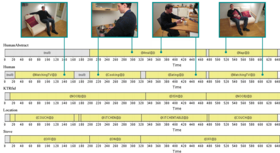
Figure 3. Evolutions in time of the components as generated by OMPS during our experiment. The plan monitoring process asserts decisions on components Human and HumanAbstract, while the RFID reader, location and stove sensor components assert decisions that reflect the sensor readings.
