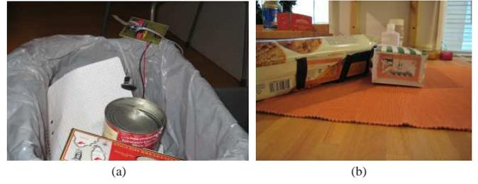
Fig. 8. Proxied objects: (a) A XBee mounted figaro proxied in garbage can. b) RFID tags under cookies and milk proxied objects.
