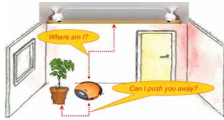
Figure 2: A simple PEIS-Ecology consisting of a vacuum cleaner, a tracking system, and a plant.
