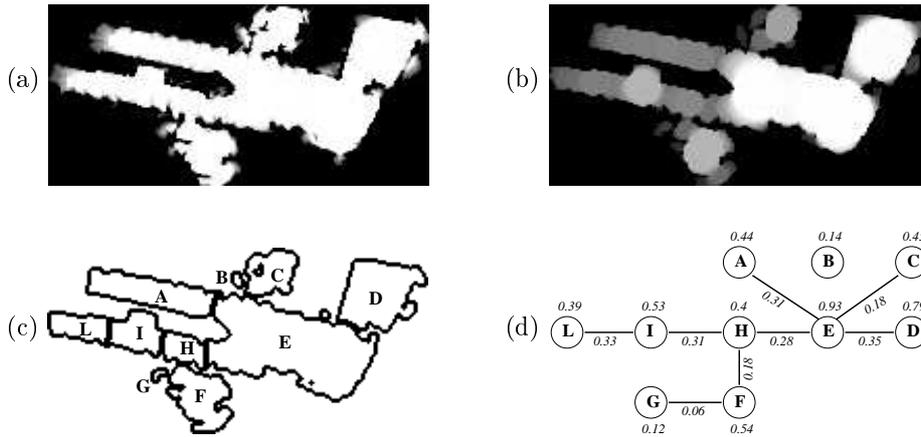
Figure 2: Extracting the topological structure of the environment from an occupancy grid by mathematical morphology. (a) Initial grid. (b) Morphological opening. (c) Connected components. (d) Adjacency graph.
