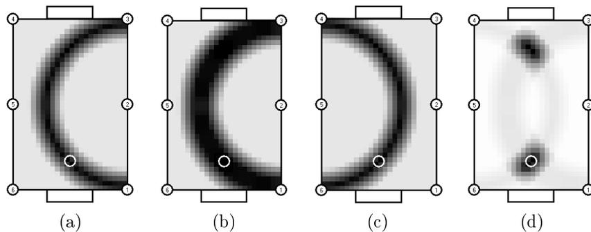
Figure 1: Self-localization on a fuzzy position grid. Darker cells have higher possibility. The white circle marks the real position of the robot. (a) The robot observes landmark number 2. (b) Fuzzy dilation after the robot moves in an unknown direction. (c) The robot observes landmark number 5. (d) The observation is fused with the existing information.
