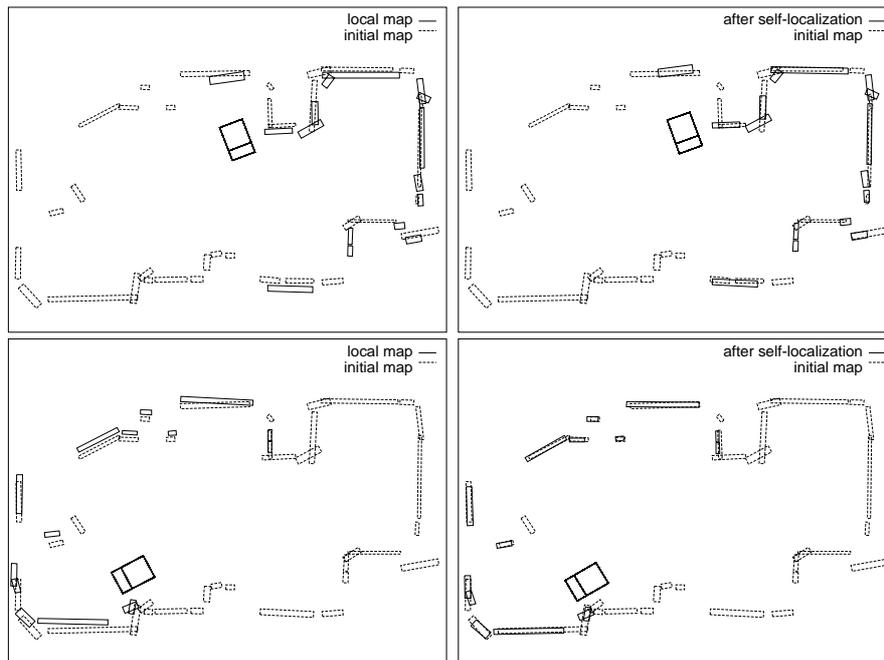
*Figure 6.* Robot self-localization at two moments during a navigation task. Left side: odometer-based position of the robot and of the local map. Right side: error correction after self-localization.
