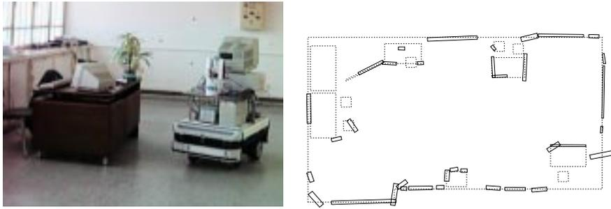
Figure 3. A view of the experimental site, and the corresponding fuzzy model (solid lines) superposed to the real map (dotted lines).
