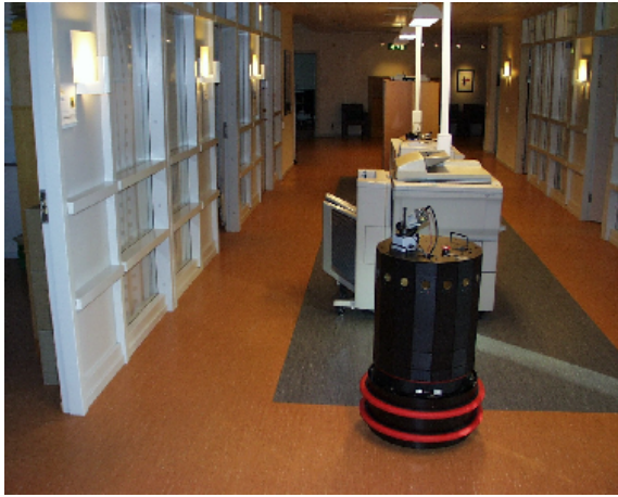
Fig. 3. The Nomad 200 mobile robot Milou and one half of the test environment (see also Fig. 4).
