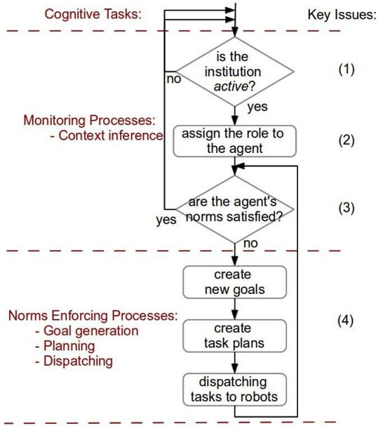
Fig. 2. How institutions are reasoned about through the four cognitive tasks. Context inference is involved in inferring if an institution is active (task 1), assigning robots to specific roles (task 2) and checking if norms are satisfied (task 3). Bringing about the adherence to norms is the purpose of goal generation and planning (task 4). In a robotic system, plans are then generated, dispatched to robots and monitored.
